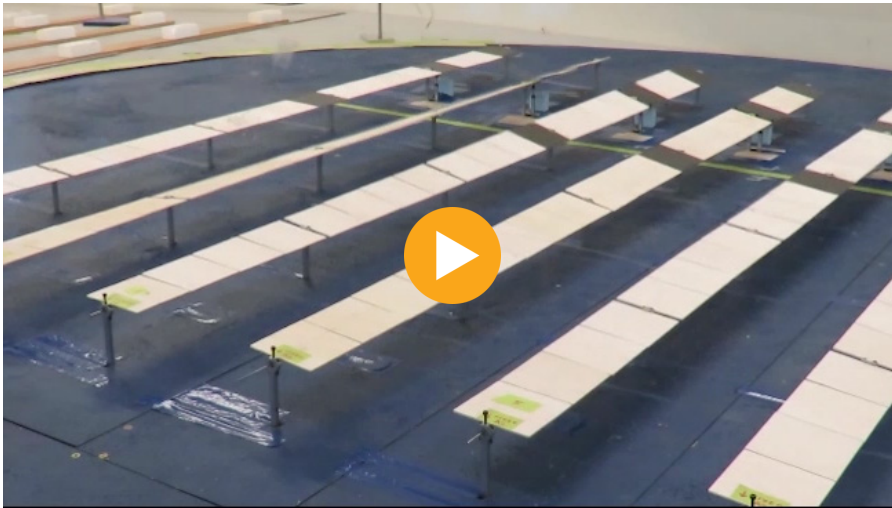
VIDEO 5: Multi-row Test of Instability at 0 Degrees (WTT) .
